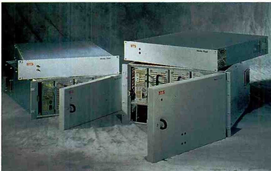
The Media Pool from BTS, a fully redundant media server developed for broadcast and post-production. Compression can be used if desired, but is not required.
