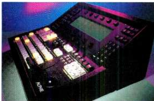
The AlphieEX, a component digital switcher capable of using virtual crosspoint technology.
